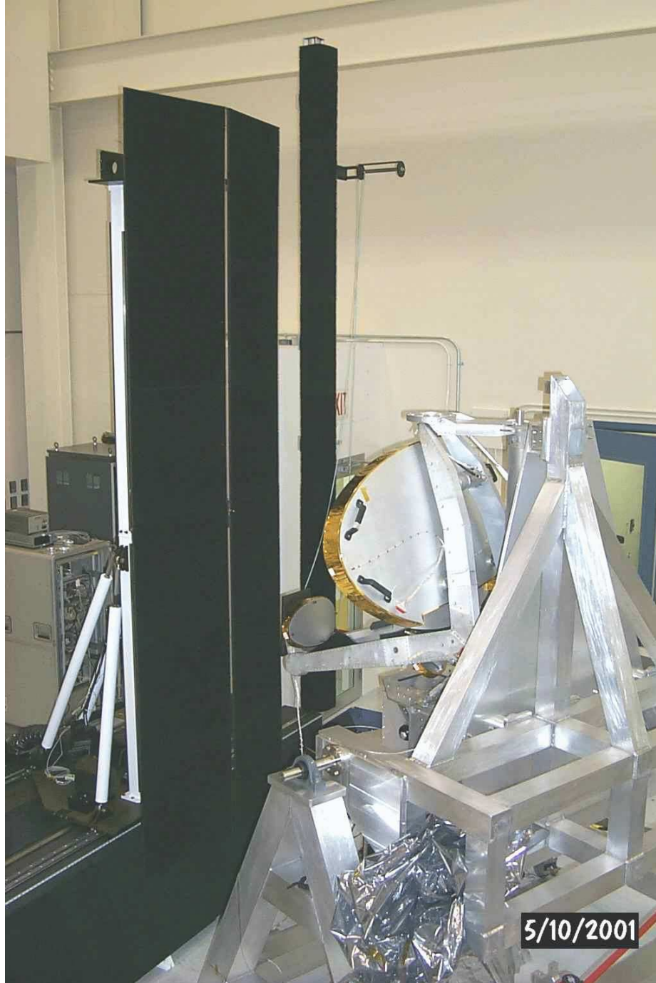
Figure D.9: Near Field Range in Building 306 High Bay Assembly and Test Facility. The black surfaces are composed of V groove absorber panels taped and tied to aluminum sheets. A probe horn is faintly visible in the gap between the 2 vertical absorber panels. This photo shows the UARS spare antenna mounted on the Field of View test fixture during initial testing of the range electronics. All of the electronics to run the testing are mounted in the gray racks behind the scanner. During flight calibrations, absorber panels cover the face of these racks. In addition, absorber panels are positioned between the scanner and the back wall of the test cell and covering portions of the FOV fixture that were observed to reflect signals back into the antenna.
