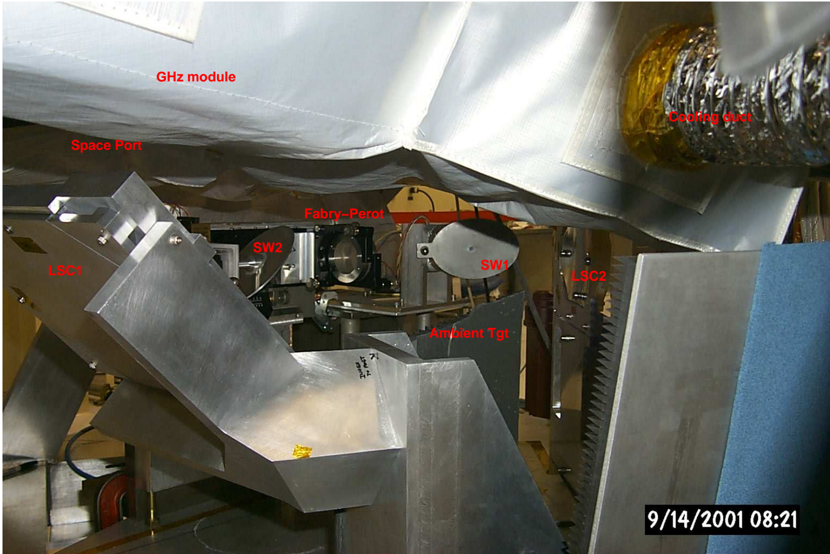
Figure 3.8: Relative Sideband calibration apparatus in the NFR configuration. See text for additional details.
